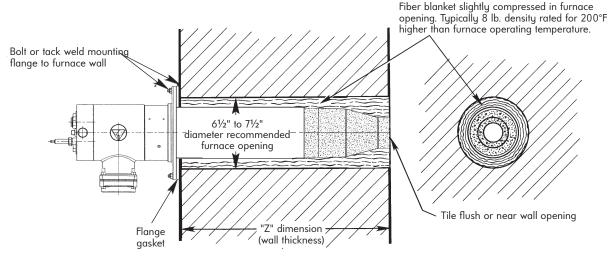
Note: If burner tile is used through an existing mounting tile, allow for 1/8" minimum clearance all around burner nozzle.
