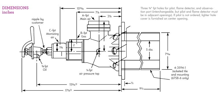
$^{\textcircled{3}}$  These dimensions assume use of a %" close pipe nipple between burner and Sensitrol Oil Valve.
