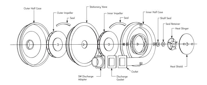
Exploded view of a hot air blower case assembly. For single stage blowers, there is no stationary vane and only one impeller.
