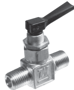
1847-03 Snap Shut Pin Valve (¼" MNPT, brass) toggle operated for quick opening or closing. Used for pneumatics, test benches, instrumentation, control panels, air lines, gauges, etc. Rated for 300 psi at 70°F; temperature limits - 40 to 200°F, Cv = 0.20.
