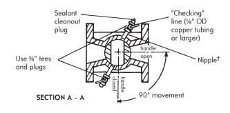
Provide 3/4" ips connecting tees and cleanout plugs between the copper tubing of the checking line and the checking connections of the FM valves. These special connections are needed to trap the sealant and prevent it from entering and eventually plugging the copper tubing, thus rendering the system inoperative. (This is a nuisance--not an unsafe failure of the system.)
