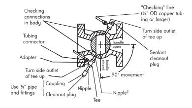
LUBRICATION REQUIRED: FM approval of 1857 Valves is valid only with Homestead #650 or #900 lubricant that is good for natural gas, propane, or coke oven gas. Use of any other lubricant voids the approval. FM requires the valves be lubricated after every 20 cycles. Lubrication is necessary for sealing and ease of operation.
