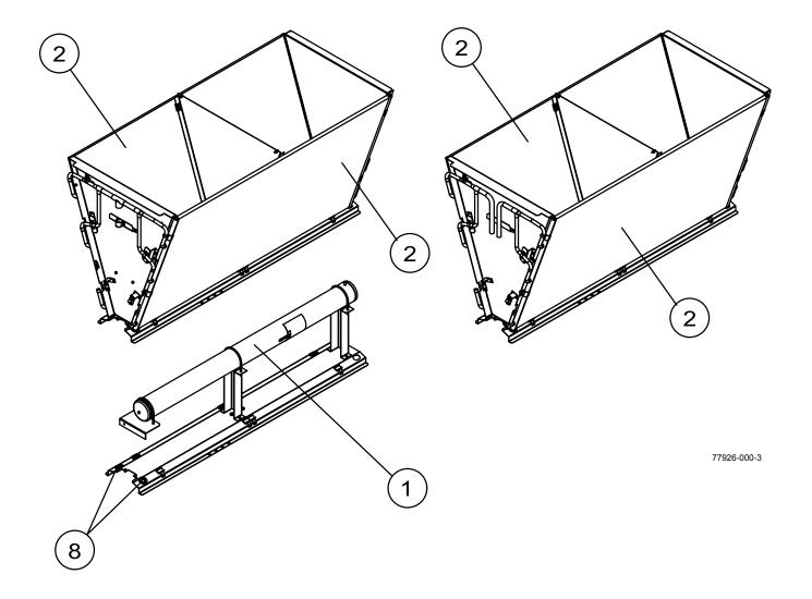
**FIGURE 1 -** MICROCHANNEL CONDENSER COIL COMPONENTS - DESIGN SERIES "A" (REFER TO TABLE 1 ON PAGE 7)
