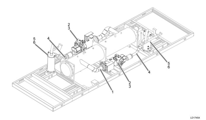
FIGURE 100 - ACOUSTICAL ARRANGEMENT, BASIC AND LEVEL 0 REDUCTION
